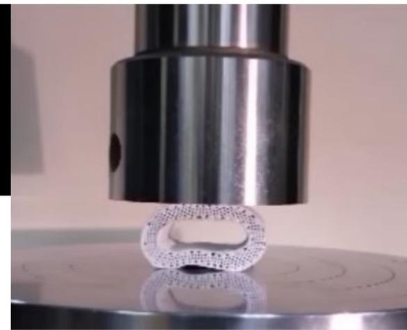
This image is showing the elasticity and durability of a structure made of hydroxyapatite.
